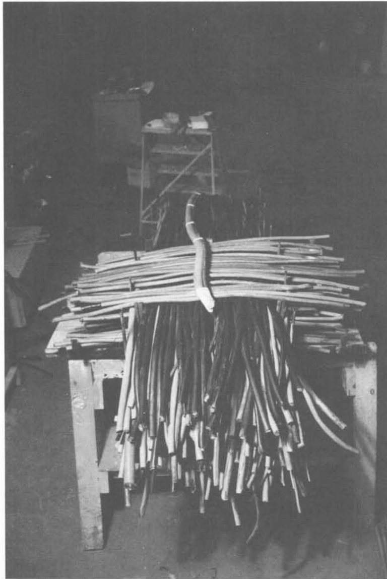
Photograph 4-11 Ignition cable on test tray bundle.
