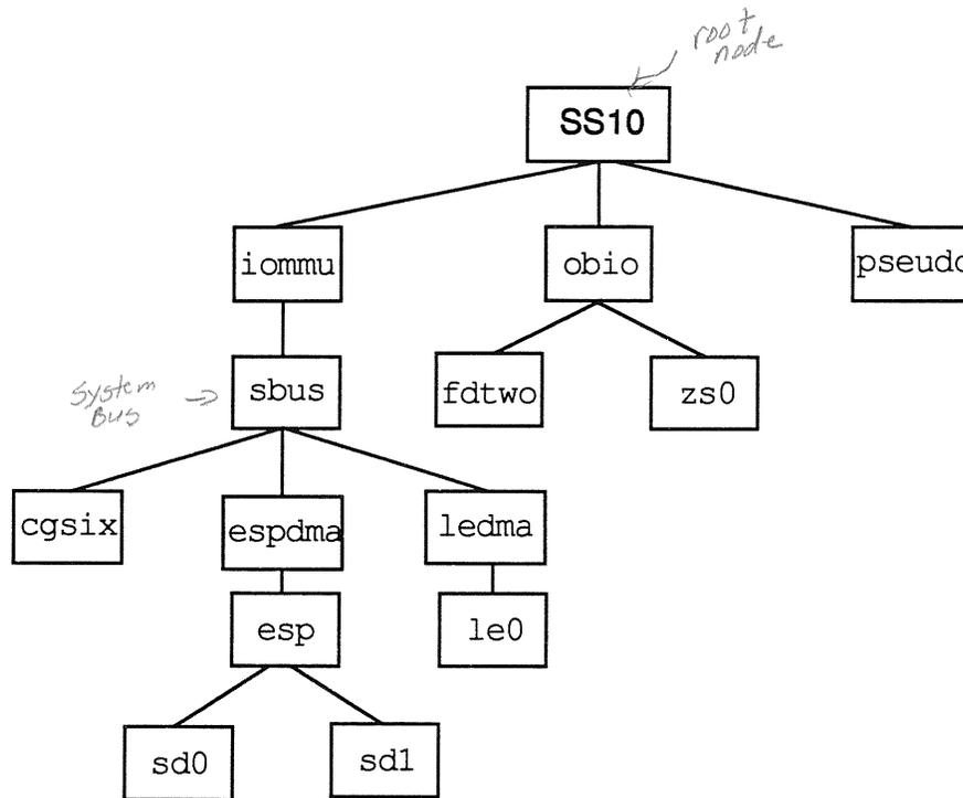
The boxes in the above diagram represent different devices on the system. For example, the `cgsix` object represents the `cgsix` color frame buffer and the `sbus` object represents the peripheral bus that is used to connect many other devices to the system.
