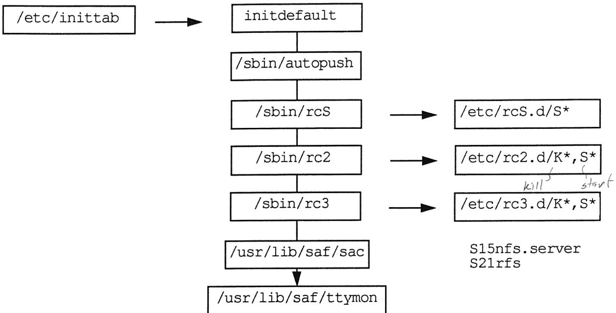
1. The `init` process looks in the `inittab` file for the `initdefault` entry, which is set to run level 3.
