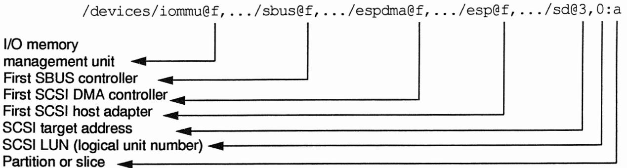
The SPARCstation 10 and newer systems have a separate I/O memory management unit (iommu) on the CPU board. The architecture of these systems also use DMA controllers for SCSI devices and ethernet devices.
