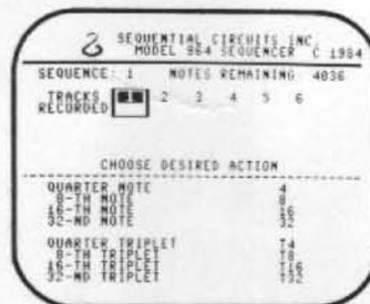
As a digital recorder, the sequencer's editing facilities allow for multi-track overdubbing, duplication, and correcting of parts without re-recording, splicing, or accumulating noise through the processes of
