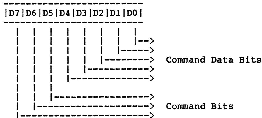
The Command Bits specify the command being issued to the 8279, and the Command Data Bits give the data associated with the command. Only three 8279 commands are used by the system software. The function of each of these commands and the definition of the corresponding data bits is as follows:
