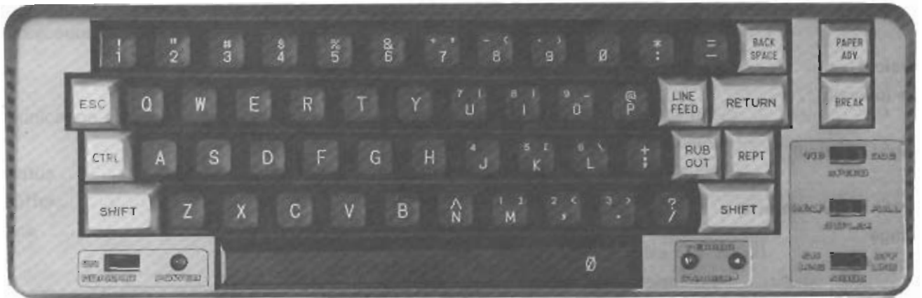
Model PT-210 Keyboard Layout and Symbolization.
