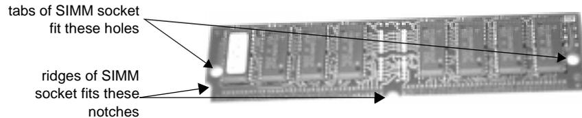
2. Gently but firmly push the module upright into the socket until the metal clips snap into place securing the module.
