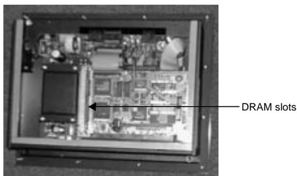
If you have a P2 PowerStation skip to the section *Removing a DRAM Module* on page 4. For all other PowerStations, you must remove the System Support card. This procedure is described on page 3.
