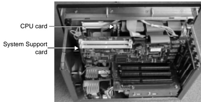
To add or replace DRAM on these PowerStations you must remove the System Support card. Follow these steps to remove the System Support card.
