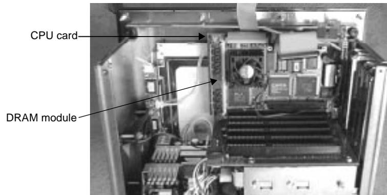
2. Push outward on the socket ejectors. It might be necessary to use a small screwdriver or the tip of a pen to push on the ejectors.
