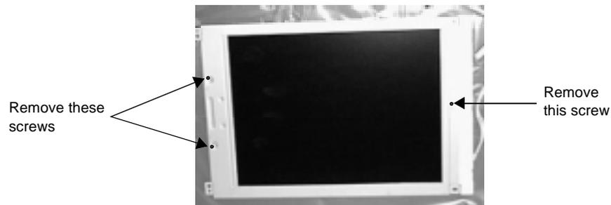
**Note** On early models, the 2 screws on the same side of the display are covered by the gasket. The gasket material covering the two screws must be removed. On later models, the gasket will be notched to allow accessibility to the screws.
