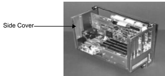
4. Install the extension plate in place of the side cover. It is easiest to pinch the extension plate from the sides and slide it into position from the top of the unit. If you have lost or misplaced the nuts that secure the side cover, the extension kit includes replacements.
