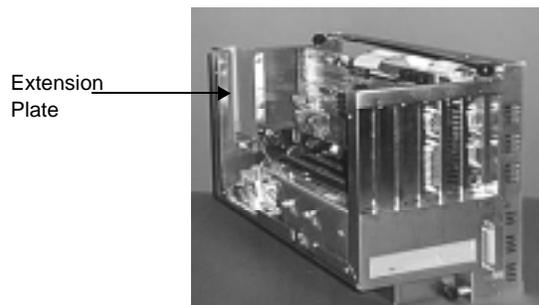
5. Remove the slot cover that corresponds to the extension plate and the appropriate slot on the back-plane board. The cover is secured by a single screw.
