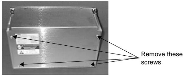
3. Remove the side cover from the left side of the PowerStation by removing the three nuts on the inside left of the unit.
