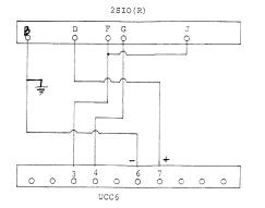
Some users report this will not work for them. They recommend the 3 P+S recommended connection. This is the more or less standard 20 mil. loop connection. If you don't have a MITS teletype, or make your connections directly to the print magnet as shown in the CC-7 manual, try this connection first.
