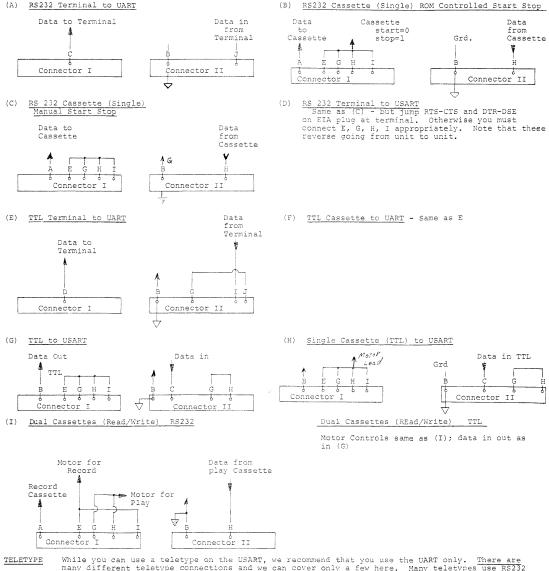
many different teletype connections and we can cover only a few here. Many teletypes use RS232 in/out hence the circuit is the same as that in (A) above. For current loop systems, typically the magnet driver (Print magnet) input is held at +5 volts
