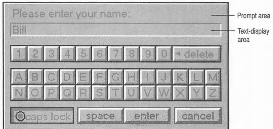
TV keyboard control with prompt and text display (KS_WITHTEXT style)
