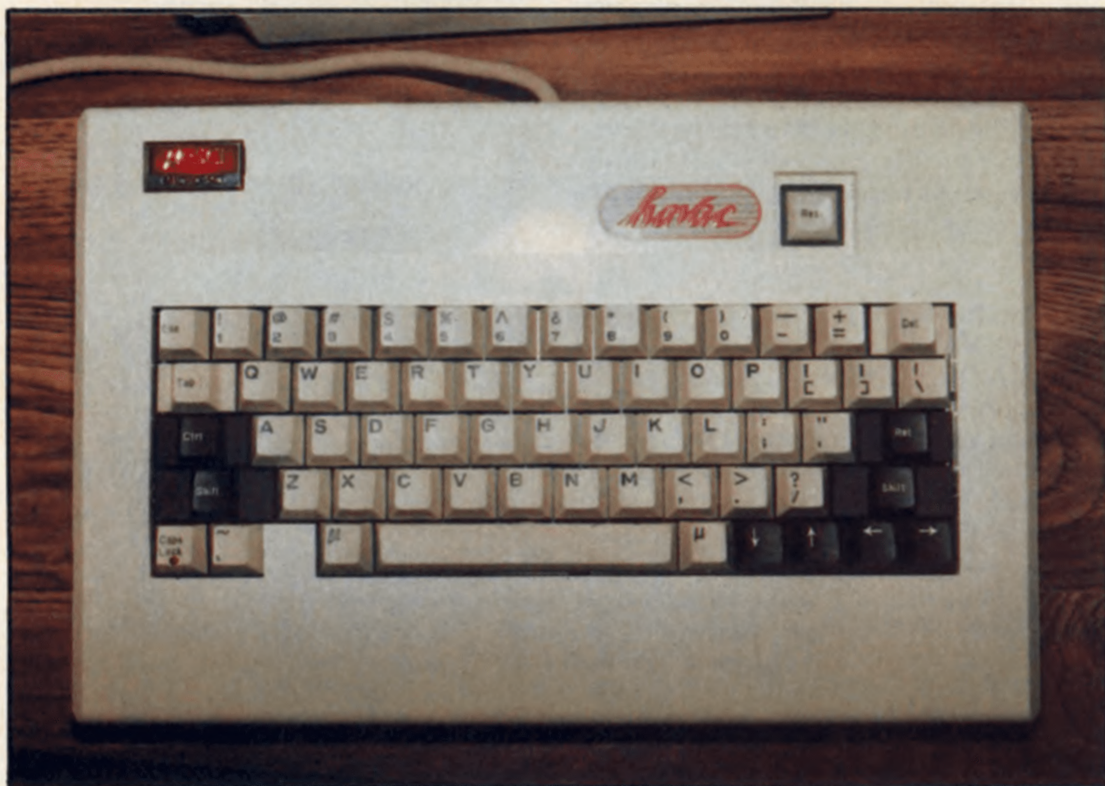
The layout of the Havac keyboard is identical to that of the Apple IIe with the exception of a small LED on the Caps Lock Key.
