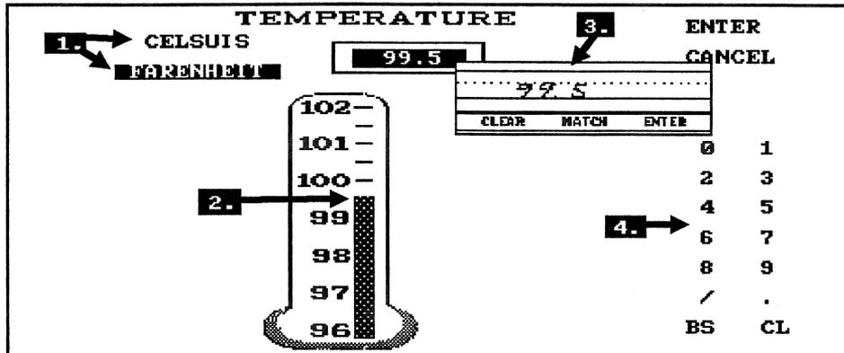
CODE-WRITE provides program access to the unique LINUS Pen-on-screen input/output routines. Four input methods are displayed: 1. Selection Buttons. 2. Point-and-enter. 3. Window for handwritten data. 4. Soft keypad.
