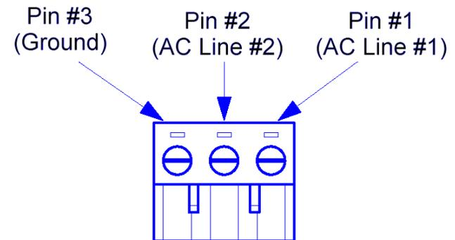
Connect the female plug to the PCB mounted AC male header. Connect the other end of the power to the AC source, taking the necessary precautions. After system mounting is complete, turn on the AC power switch.
