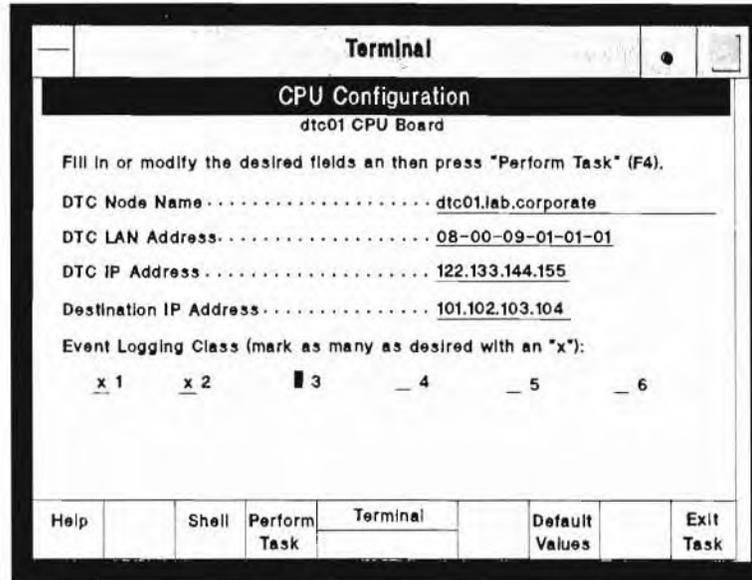
The screenshot shows a terminal window titled "Terminal" with a "CPU Configuration" screen for "dtc01 CPU Board". The screen prompts the user to "Fill in or modify the desired fields and then press 'Perform Task' (F4)". The configuration fields are as follows:
