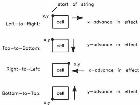
**Figure 3-1. Character Positioning at x,y Coordinates.**
