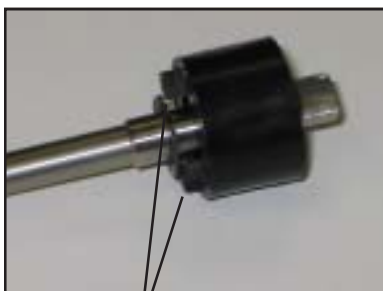
Tabs in Brake Roller Shaft
