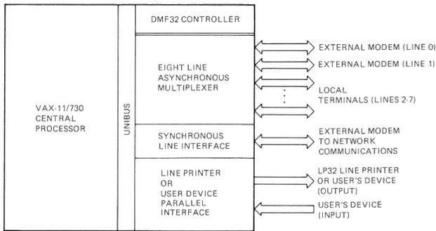
The general purpose interface transfers 16-bits of data between a user specific device and the VAX-11/730 system. The signal levels are TTL compatible.
