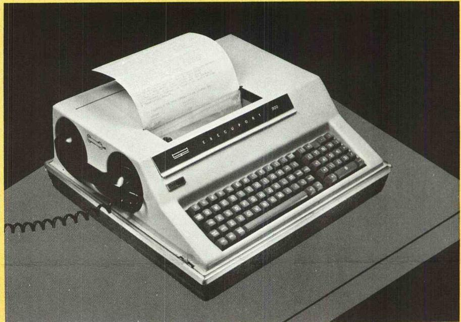
**MODULAR CONSTRUCTION** provides quick, easy functional expansion through the addition of visual display and tape "memory" plug-in units.
